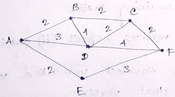
Step 3:- Suppose source vertex is A, and destination vertex F. Now we find out the shortest path from A to F.
